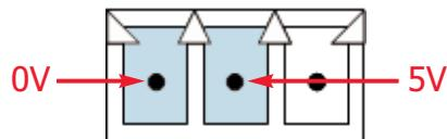
If the control **can** supply the required power, insert the link provided as shown below.
